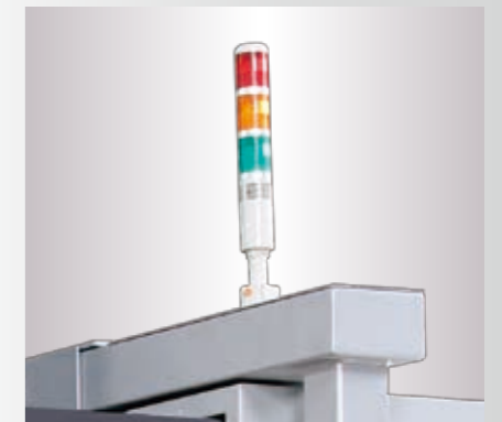
Operation cycle finish and alarm lights (STD)
